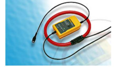
The i3000s Flex is an ac current clamp utilizing the Rogowski principle. It can be used to measure currents up to 3000 A when used in conjunction with oscilloscopes, recorders or data loggers. The flexible and lightweight measuring head allows quick and easy installation in hard to reach areas.
