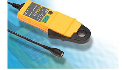
The i310s current probe is based on Hall Effect technology for use in measurement of both DC and AC current. The i310s may be used in conjunction with oscilloscopes and other suitable recording instruments for accurate non-intrusive current measurement.
