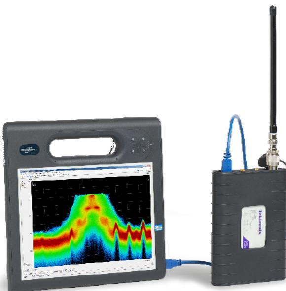
While it's very important to determine frequency, occupied bandwidth and relative signal strength; we also need to find out how often a signal is on.
