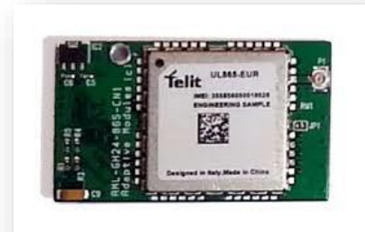
MCU, Wireless module Crystal, antenna, voltage regulators, balun, shielding, Passives, etc.
