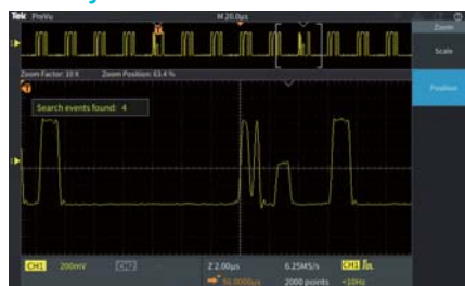
Search and Mark features for easy identification of events that occur in the acquired waveform
