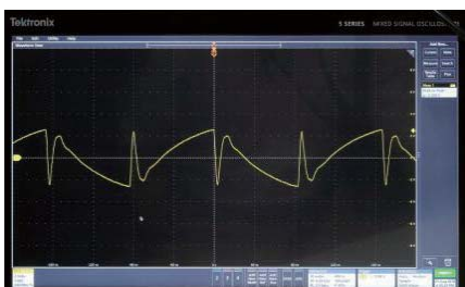
Waveform on Oscilloscope. DUT impedance impacts the waveform.
