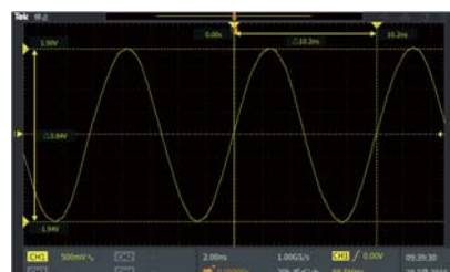
Innovative cursor measurements with on-waveforms readouts
