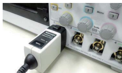
TekVPI probes communicate scale settings, ranges, and status to the TBS2000B
