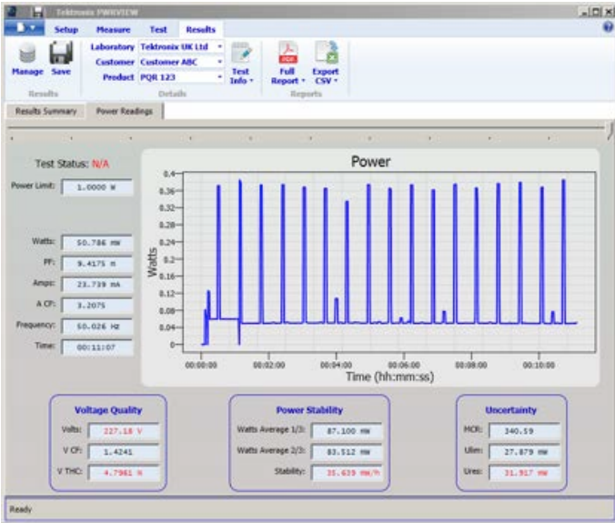
Figure 33. Tektronix PWRVIEW standby power measurement.
