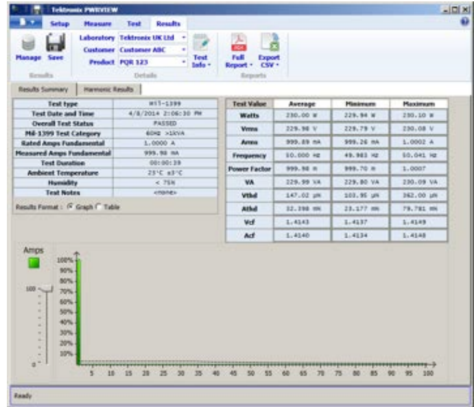
Figure 34. PWRVIEW PC software charts harmonics and compares to limits.
