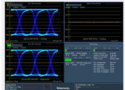
Eye and Jitter display, along with automated measurements of physical layer parameters
