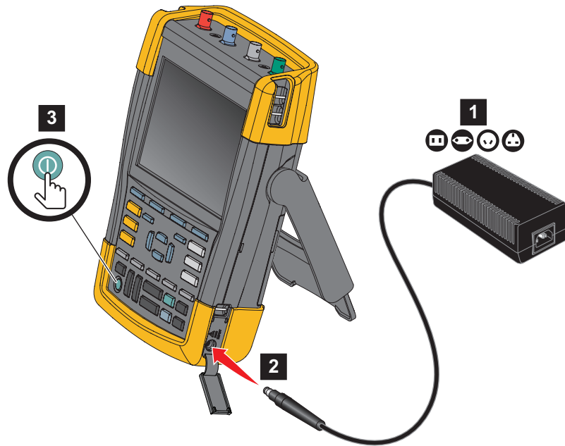
Figure 1. Powering the Test Tool
