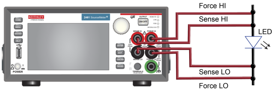
Figure 57: Model 2461 4-wire connections to the front panel
