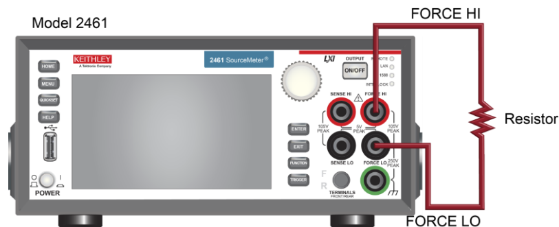
Figure 19: Model 2461 2-wire front-panel connections
