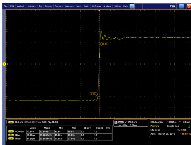
Figure 14: P77STFLXA solder tip attached with 75 mils (1.90 mm) wires (rise time = 27.9 ps)
